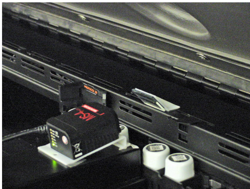
Figure 7-15. Bar Code Reader Option and Sample Vials with 2D Bar Codes on Vial Caps.
